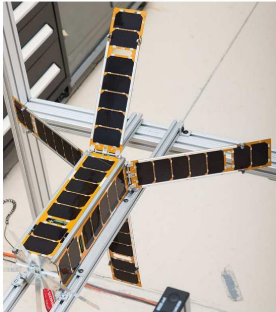
Figure 3: Example of nitinol alloy for the satellite panel opening system using 4D printed hinges
