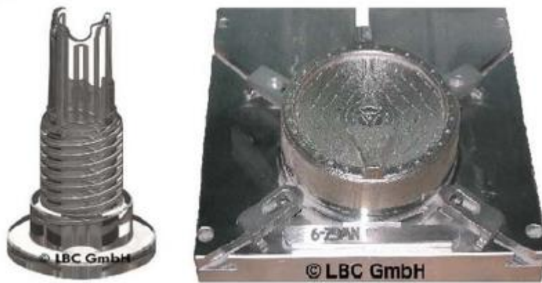
Figure 2: Examples of application of 3D printing for machine tool parts
